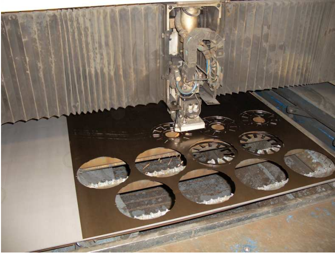
Figure 8.8: Laser cutting of the stator and translator iron laminations.
