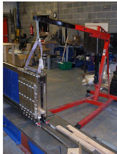
Fig. 15. Mounting the c-core modules using an engine hoist
